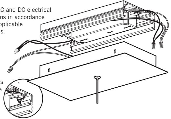
5. Attach the canopy plate and cover assembly to the base using screws.
