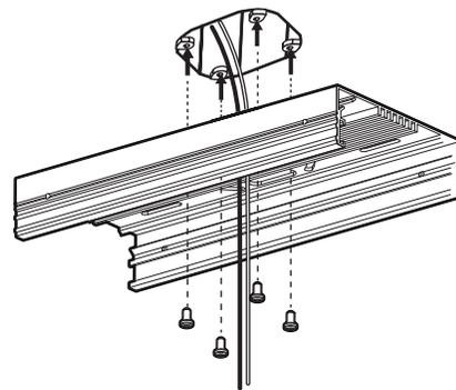
2. Install the transformer into the base profile, using M4 screws, on top of the longitudinal channels.
