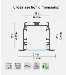
The ultimate in simplified LED lighting! The 8500 recessed profile is designed for use with standard and HOS LED engines. With its elegant and discreet edges, the 8500 fits perfectly and requires no plastering. Its ingenious design includes Type B grooves that allow the use of flat and 45°/135° joiners, ideal for angled fittings. It is a masterpiece in terms of ease of installation, luminous intensity and creative set-up.
