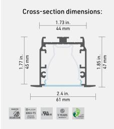
The ultimate in simplified LED lighting! The 8500 recessed profile is designed for use with the LuxLine 120 V LED engine. With its elegant and discreet edges, the 8500 fits perfectly and requires no plastering. Its ingenious design includes Type B grooves that allow the use of flat and 45°/135° joiners, ideal for angled fittings. It is a masterpiece in terms of ease of installation, connection and creative set-up.
