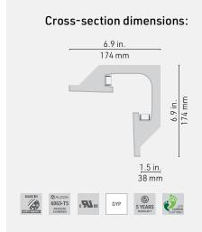
GEMINUS creates **corner alcoves** with a 2-inch wide opening, uniformly lit from both sides, for a more emphasized linear lighting effect. A direct fit for 1/2-inch gypsum panels, it can also be leveled with 5/8-inch ones, with the same ease of installation and effectiveness as with other Gypsum Series profiles.
