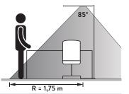
When presence detected, the luminaire switches on immediately. Detection angle 85°
