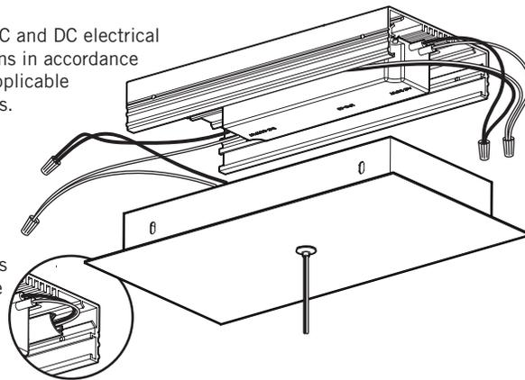
5. Attach the canopy plate and cover assembly to the base using screws.
