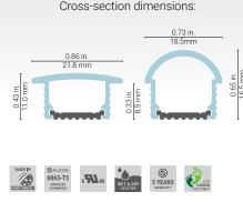
The 5000 consists of an **aluminum heatsink base** inserted into a **flexible recessed lens** with gripping sides. It allows for a very **simple installation**, with the assembly inserted into the recess and staying in place due to the gripping ribbed lens sides. The 5/8" wide and 3/8" deep recess is a direct fit for North American cabinetry, closet, or mural applications, besides being economical and providing lighting without hot spots.
