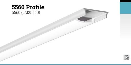
The 5560 profile allows integrating linear LED lighting on **curved or uneven surfaces**. Its low profile (1/5" including lens), and a thickness of less than 1/32" (0.75mm), allows for **effort-less bending and installation** using plain mounting tape or screws. The opal lens will provide a diffused light effect without harsh dots.
