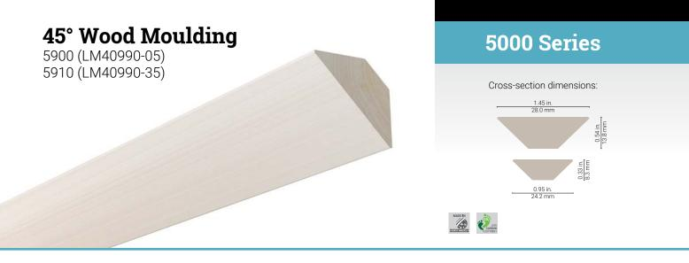
The **limewood 45-degree mouldings** are the woodworker's solution to integrating linear LED lighting in furniture, cabinetry, or other locations having inside corners. Available in widths of 1.5" to accomodate stronger LED lighting in an aluminium profile, and 1" for an exposed LED strip on a basic heatsink. The back clearance allows passing and concealing the electrical wiring. Its smooth surface can be tinted, primed and painted.
